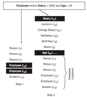
Fig.5. Steps of database stack during processing queries.
